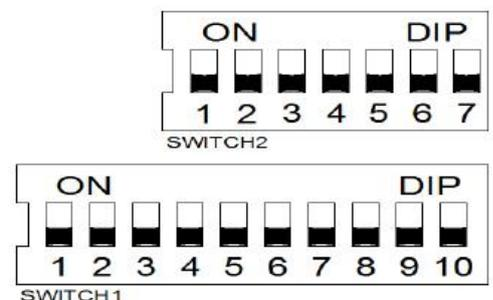
Sensitivity and frequency of the loop can be adjusted by 7-way dip switch and 10-way dip switch setting.
