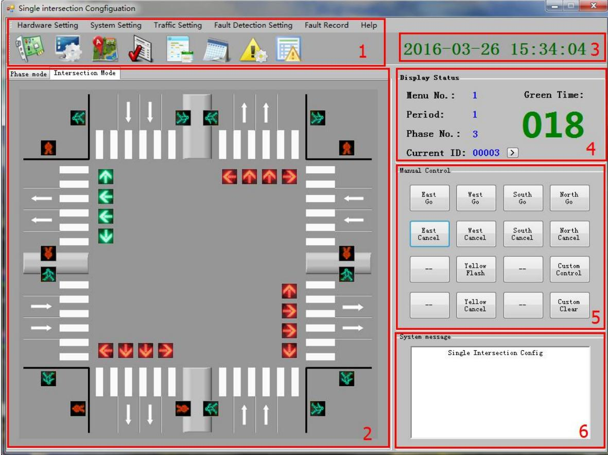
Figure 6 Single Intersection Configuration (Intersection Mode)
